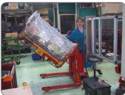
The straddle model makes it possible to handle closed pallets. The Ergo-Tilt being used in the component industry.
