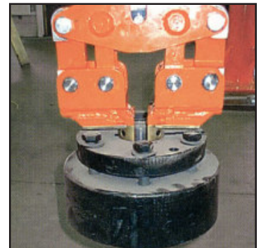
Tool handles a 150-pound wheel hub assembly by gripping the inside diameter of the hub and orienting the hub to a tire rim
