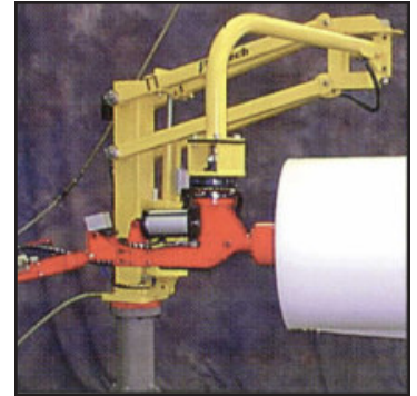
This core gripper on a World Manipulator allow for easy handling of bulky rolls of paper, plastic and film in doffing, palletizing, and crating operations
