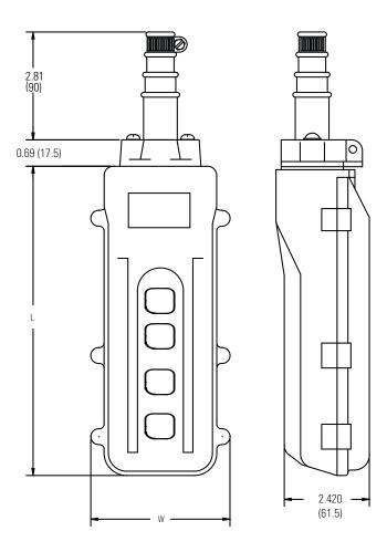
The CM LodeStar Control Station Pendants feature a compact, ergonomic design with the operator's comfort in mind. They are available with 1, or 2 speed buttons. It is equipped to accommodate either internal or external strain relief cable.
