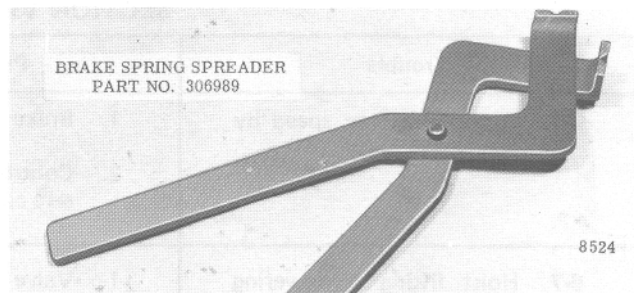
Figure 7-4. Special Tool for Removing Brake Spring.
