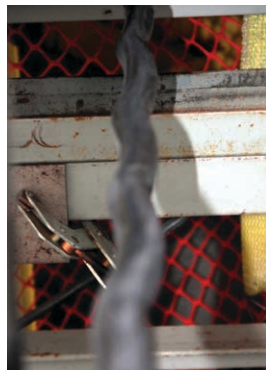
Failing cable due to the “corkscrew” effect
