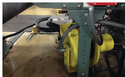
Failing cable due to the “corkscrew” effect
