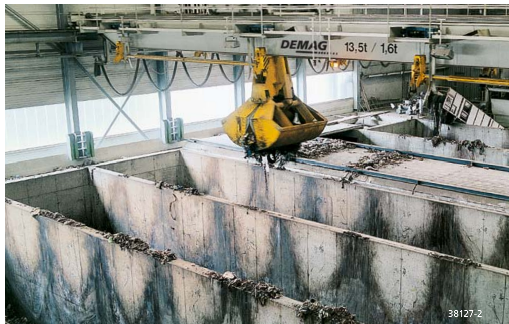
Demag Process Cranes used for fully automatic filling of composting boxes with residual waste in a waste disposal installation
