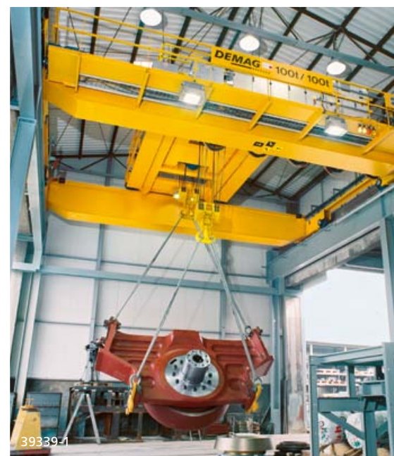
Cranes are used for turning components in the production of crusher parts
