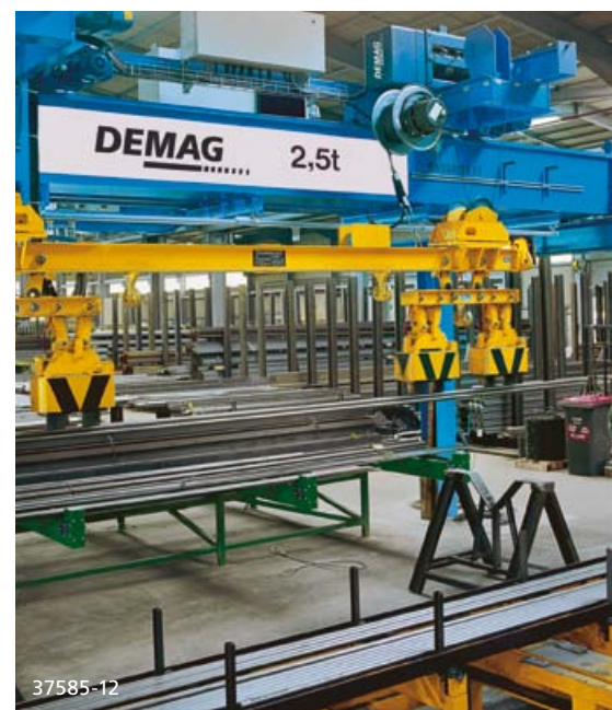
Demag Coilmaster in a fully automatic coil store with magnets or grabs as load handling attachments
