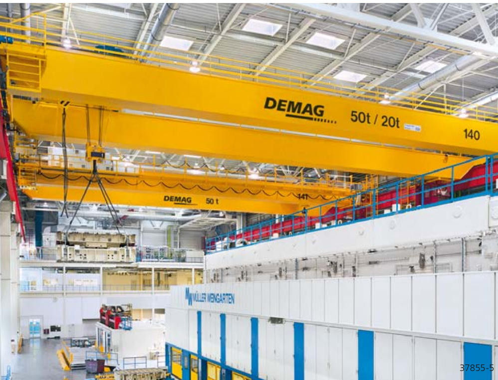
Demag Process Cranes changing tools in a press plant in the automotive industry
