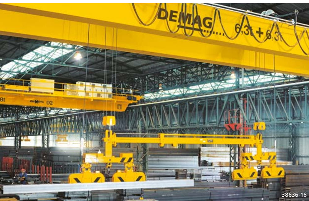
Demag Steelmaster with a magnet spreader for handling long materials, single items or metal plates
