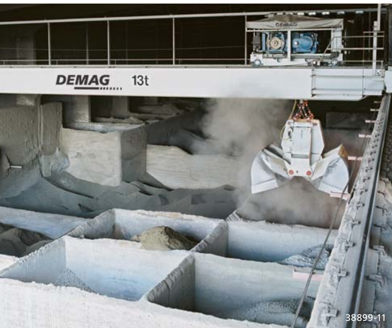
Fully automatic replenishment and retrieval of the various additives by a Demag automatic crane in a cement works
