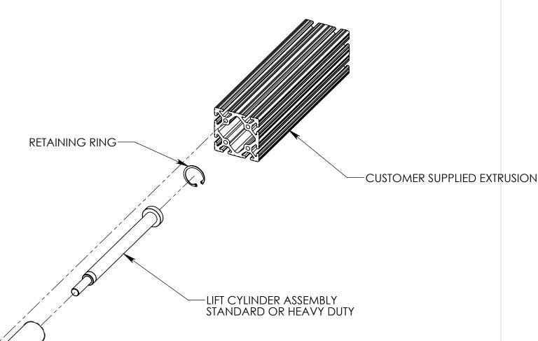
INTERNAL HOUSING ASSEMBLY CONTAINS SUPPORT TUBE AND LIFT CYLINDER-
