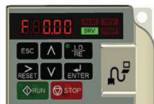
Figure 7: G+ Mini Digital Operator Main Display
