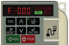
Figure 3: G+ Mini Digital Operator Power-up State
