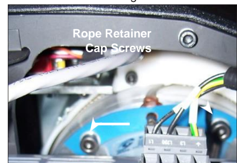
Diagram T. Remove the two M8 socket head cap screws and slide retainer off of rope end towards you. Configuration may vary depending on capacity.
