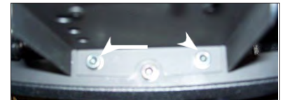
Diagram P. Remove (4) M5 SHCS (2 on top and 2 on bottom) that fasten the swiveling PCB bracket to the front support plate.
