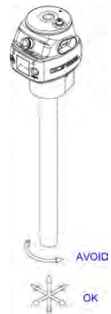
Diagram 6E3. Proper use of Force Sensing Handle grip.
