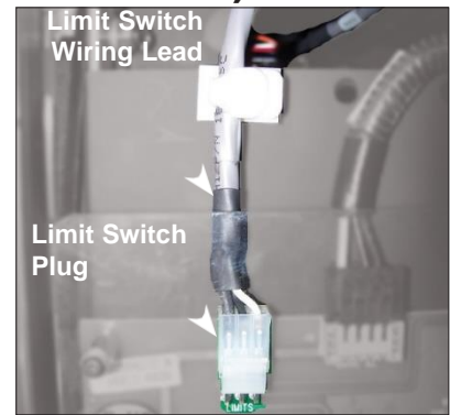
Diagram P. Gently pull out the grey limit switch wiring lead to disconnect plug from board.
