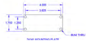
Diagram 6F2. Mounting plate dimensions.
