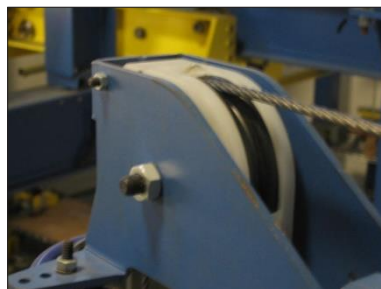
Diagram V. Pulley block at end of arm.
