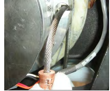
Diagram T. Insert rope from actuator through opening at bottom & form loop to set in radius channel
