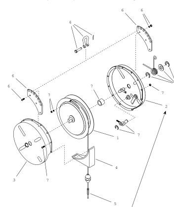
NOTE: / \*When ordering Right Hand Housing Assembly (REF NO. 2) for LOCKING MODELS, you must add "–L" to the kit number.
