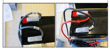
The newly installed batteries should be positioned as shown. • Replace the battery compartment cover.
