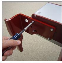
3) Position the axle and any other cross piece through the appropriate location hole in the mounted foot. Place the free
