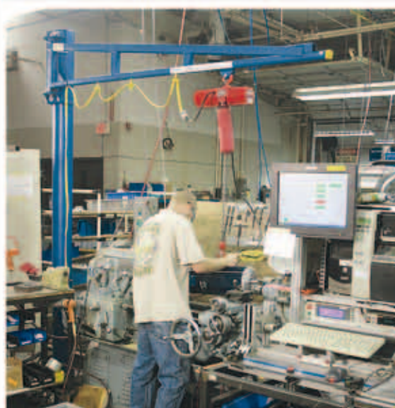
Floor Mounted TSJ150 in motor assembly area with light duty chain hoist
