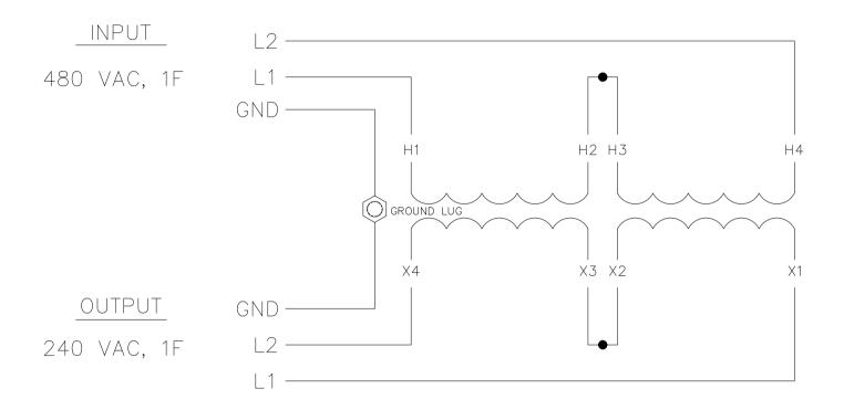
NOTE 1: THE ABOVE WIRING REFLECTS THE PROPER CONFIGURATION FOR 480-240 STEP-DOWN ONLY.
