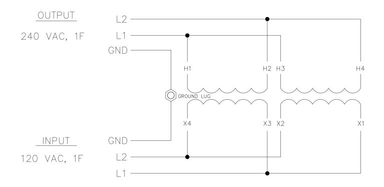
NOTE 1: THE ABOVE WIRING REFLECTS THE PROPER CONFIGURATION FOR 120-240 STEP-UP ONLY.
