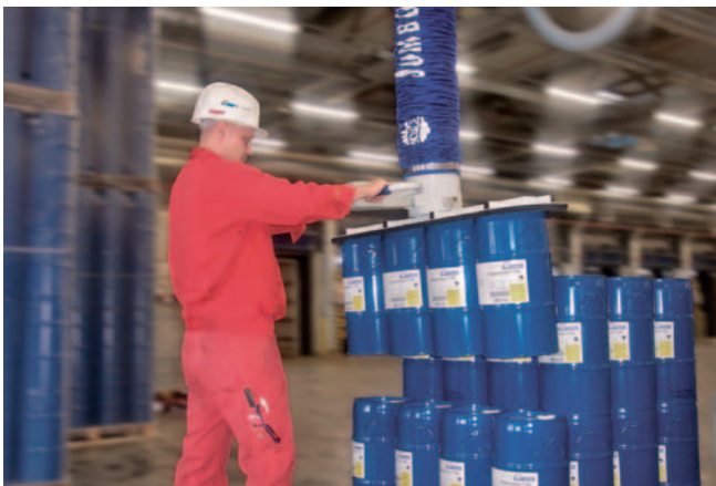
JumboErgo, maximum load 140 kg, with customer-specific gripper solution, for simultaneous handling of four barrels
