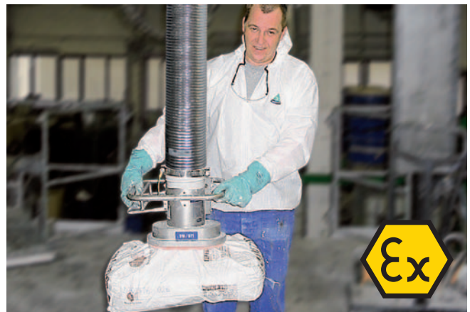
JumboSprint, maximum load 65 kg, with sack gripper, for handling sacks in explosion-proof areas to ATEX
