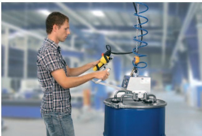
VacuMaster Eco, maximum load 250 kg, horizontal, for handling of barrels
