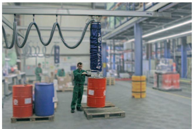
JumboErgo, maximum load 300 kg, with round suction pad, for handling barrels
