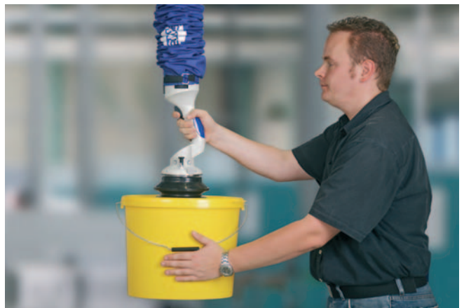
JumboFlex, maximum load 35 kg, with round suction pad, for handling of buckets
