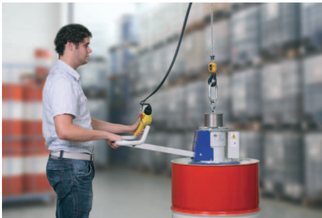
VacuMaster Eco, maximum load 250 kg, horizontal, for handling of barrels
