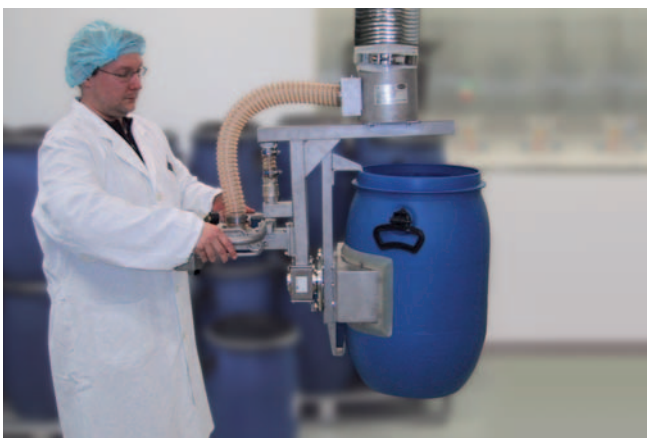
JumboErgo, maximum load 85 kg, with side gripper, for handling and emptying barrels
